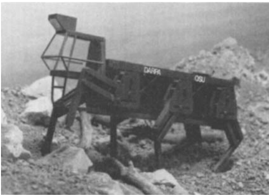
FIGURE 47.4 The adaptive suspension vehicle ( 1/10 -scale model). This is a vehicle for transportation in very rough terrain conditions which uses legged locomotion. ( The Ohio State University. )
