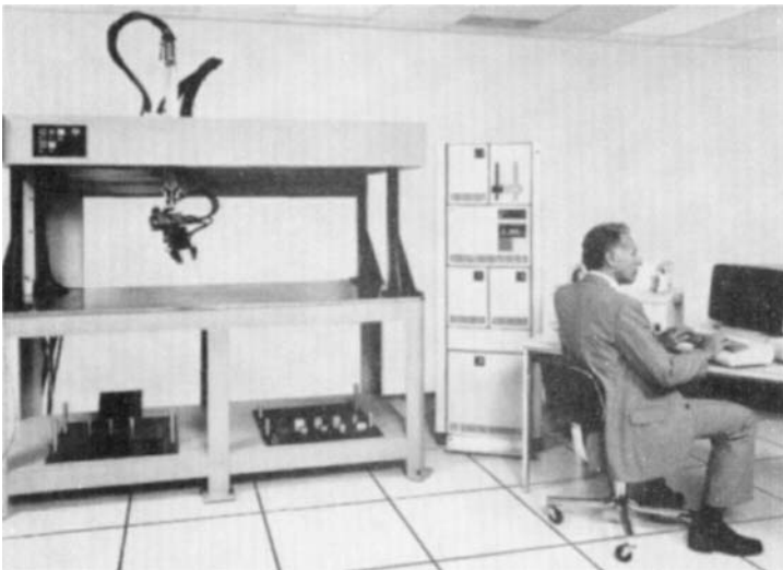
FIGURE 47.6 Robot suitable for assembly operations. Orthogonal slide arrangement gives uniform positioning accuracy and is well adapted to planar transport of parts and unidirectional insertion. Large range of motion in wrist and force-sensing gripper gives good dexterity.
