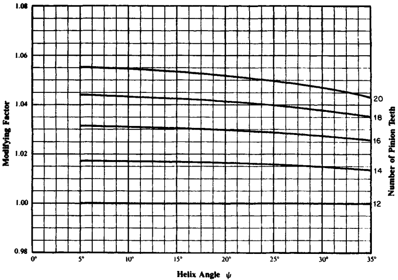
FIGURE 35.36 J factor multipliers for 20° normal-pressure-angle helical gears with short addendum (75 percent of standard). These factors can be applied to the J factor when other than 75 teeth are used in the mating element. (From Ref. [35.1].)
