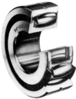
FIGURE 27.3 Rolling bearing with spherical rolling elements to permit misalignment up to \pm 3^\circ with an unsealed design. The sealed bearing, shown above, permits misalignment to \pm 2^\circ . ( McGill Manufacturing Company, Inc. )
