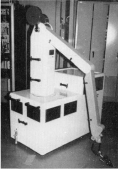
FIGURE 47.7 Manipulator for use by quadriplegic. This device is a teleoperator which operates from very limited inputs and achieves good accuracy despite light, compliant structure and drive because operator's vision provides endpoint feedback. ( Jean Vertut, CEA, Saclay, France. )
