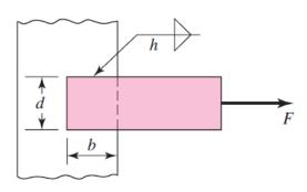
**9-1** Given, b = 50 mm, d = 50 mm, h = 5 mm,  $\tau_{\text{allow}} = 140$  MPa.
