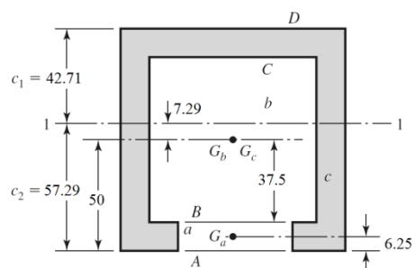
$$\bar{y}_a = 6.25 \text{ mm}, \bar{y}_b = 50 \text{ mm}, \bar{y}_c = 50 \text{ mm}$$
