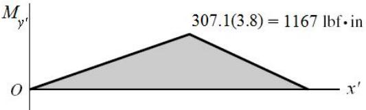
(c) The critical stress element is just to the right of  $Q$ , where the bending moment in both planes is maximum, and where the torsional and axial loads exist.
