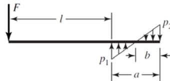
$$q = -F \langle x \rangle^{-1} + p_1 \langle x - l \rangle^0 - \frac{p_1 + p_2}{a} \langle x - l \rangle^1 + \text{terms for } x > l + a$$
