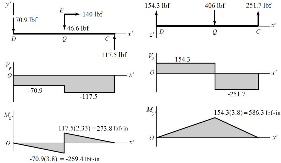
(c) The critical stress element is just to the right of  $Q$ , where the bending moment in both planes is maximum, and where the torsional and axial loads exist.
