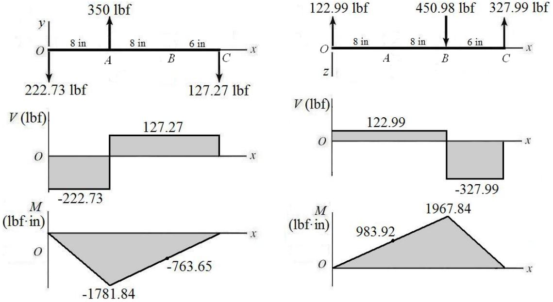
(d) Combine the bending moments from both planes at *A* and *B* to find the critical location.
