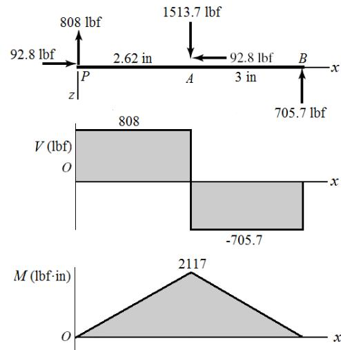
**(c)** The critical stress element is just to the left of  $A$ , where the bending moment in both planes is maximum, and where the torsional and axial loads exist.
