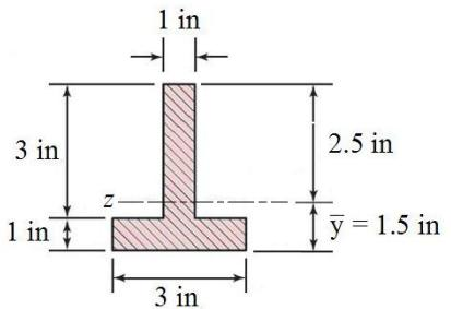
$$\text{At } x = 10 \text{ in}, \quad y = -1.5 \text{ in}, \quad \sigma_x = -\frac{-18000(-1.5)}{8.5} = -3176 \text{ psi}$$
