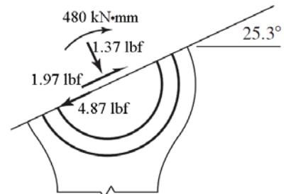
On the surface  $25.3^\circ$  from the horizontal, find the internal forces in the tangential and normal directions. Resolving  $F_1$  into components,
