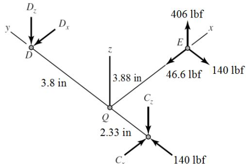
(b) For  $DQC$ , let  $x', y', z'$  correspond to the original  $-y, x, z$  axes.
