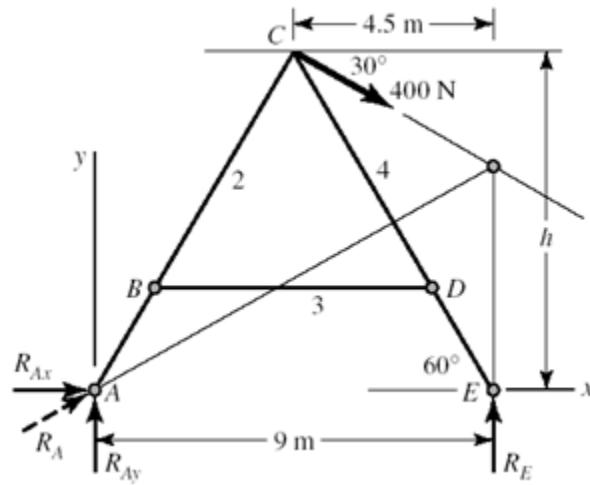
Step 2: Find components of  $R_C$  on link 4 and  $R_D$
