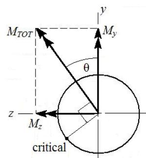
The combined bending moment vector is at an angle of  $30.3^\circ$  CCW from the  $y$  axis. The critical bending stress location will be  $90^\circ$  CCW from this vector, where the tensile bending stress is additive with the tensile axial stress. The critical stress element is therefore on the outer surface, at an angle of  $30.3^\circ$  CCW from the  $z$  axis.
