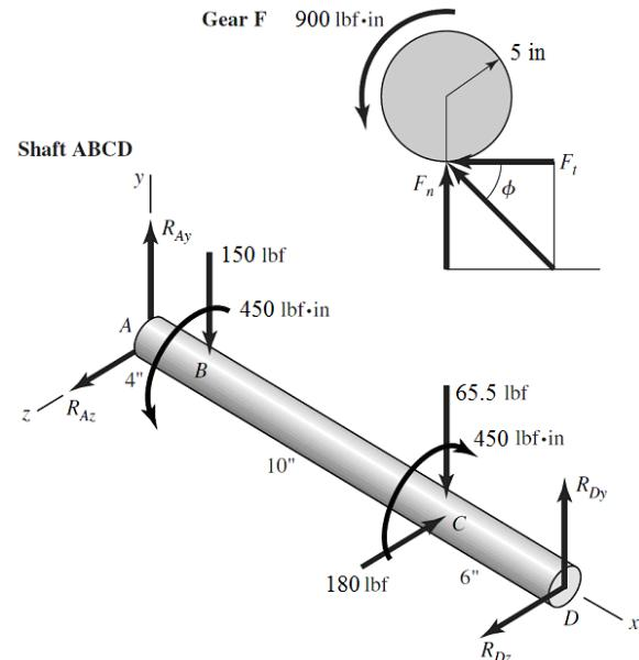
$$\sum(M_A)_z = 0 = 20R_{Dy} - 65.5(14) - 150(4) \Rightarrow R_{Dy} = 75.9 \text{ lbf}$$
