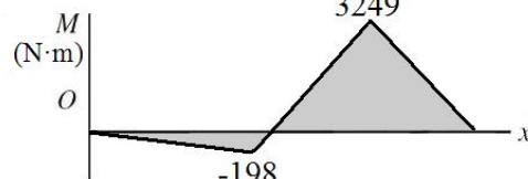
(d) From the bending moment diagrams, it is clear that the critical location is at B where both planes have the maximum bending moment. Combining the bending moments from the two planes,
