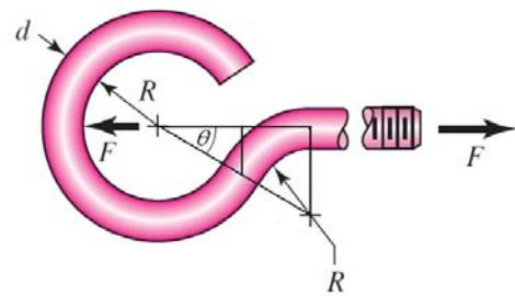
**3-124**  $d = 0.25 \text{ in}$ ,  $r_i = 0.5 \text{ in}$ ,  $r_o = 0.75 \text{ in}$
