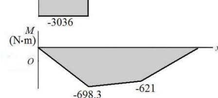
**(d)** The maximum bending moment is at  $x = 230$  mm, and is  $M = -698.3$  N·m. Since the shaft rotates, each stress element will experience both positive and negative bending stress as it moves from tension to compression. The torque transmitted through the shaft from  $A$  to  $B$  is  $T = (1800 - 270)(0.200) = 306$  N·m. For a stress element on the outer surface where the bending stress and the torsional stress are both maximum,
