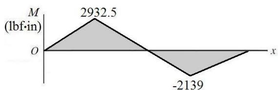
**(d)** The maximum bending moment is at  $x = 10$  in, and is  $M = 2932.5$  lbf·in. Since the shaft rotates, each stress element will experience both positive and negative bending stress as it moves from tension to compression. The torque transmitted through the shaft from  $A$  to  $B$  is  $T = (500 - 75)(4) = 1700$  lbf·in. For a stress element on the outer surface where the bending stress and the torsional stress are both maximum,
