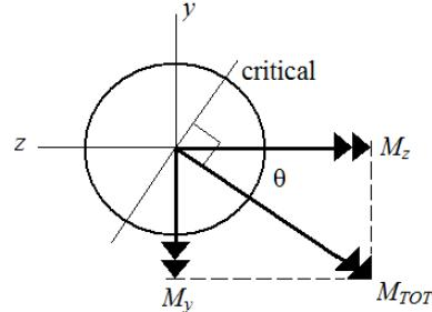
The combined bending moment vector is at an angle of  $36.3^\circ$  CW from the negative *z* axis. The critical bending stress location will be  $\pm 90^\circ$  from this vector, as shown. Since there is an axial stress in tension, the critical stress element will be where the bending is also in tension. The critical stress element is therefore on the outer surface at the wall, at an angle of  $36.3^\circ$  CW from the *y* axis.
