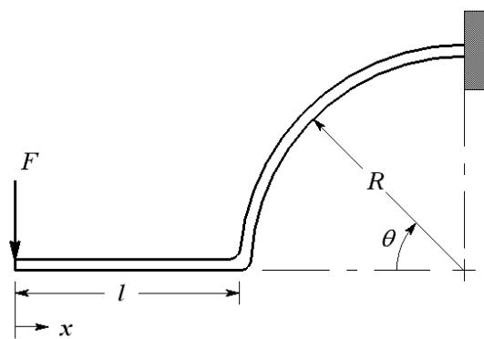
$$M = -Fx, \quad \frac{\partial M}{\partial F} = -x \quad 0 \leq x \leq l$$
