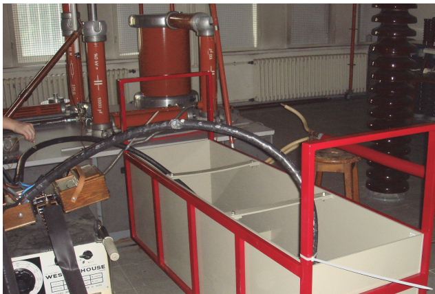
Fig. 15. Experimental set-up for 0.6/1 kV cable.
