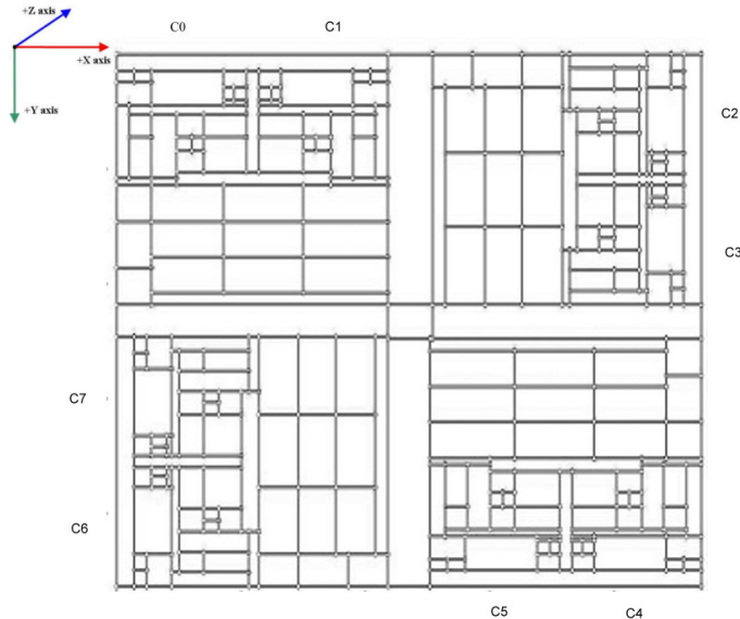
Fig. 9. The extracted IBM POWER4 MCM floor plan
