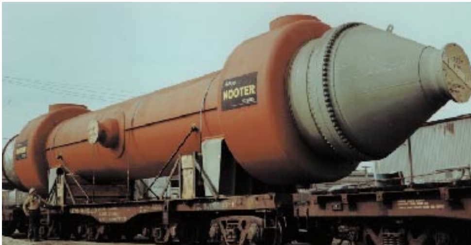
PLATE 10 Pressure vessel. (Photo courtesy Nooter Corp., St. Louis, MO.)
