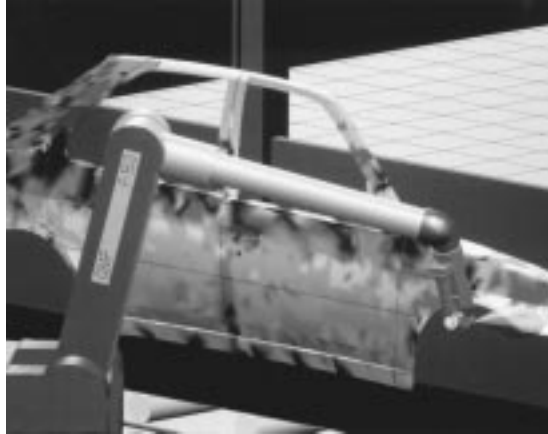
FIGURE 14.11.4 Painting operation simulated in off-line programming environment. Estimated paint thickness is illustrated by shading. (Courtesy of SILMA, Inc.)
