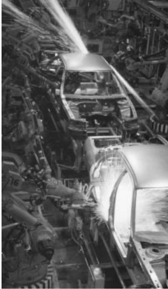
FIGURE 14.11.1 Six-axis articulated arm robots spot weld automobile bodies on a transfer line. (Courtesy of Nachi Robotics, Ltd.)
