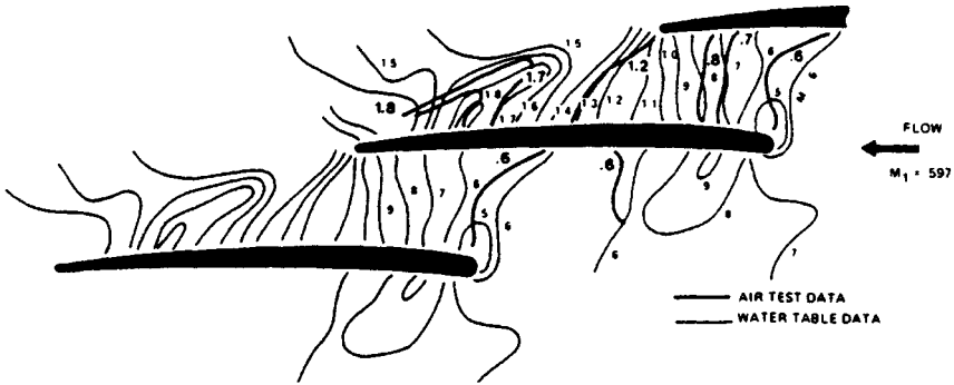
Fig. 58.42 Comparison of water table test results with interferometry air test data for Mach number distribution in transonic blade.
