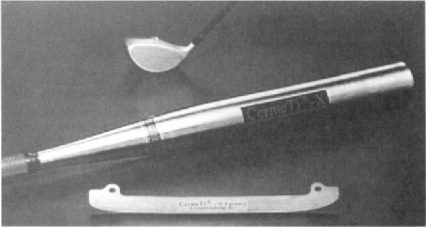
Fig. 9.33 Developmental sports equipment using titanium carbide particle-reinforced titanium, including a golf club head, bat, and ice skate blade (courtesy Dynamet Technology).
