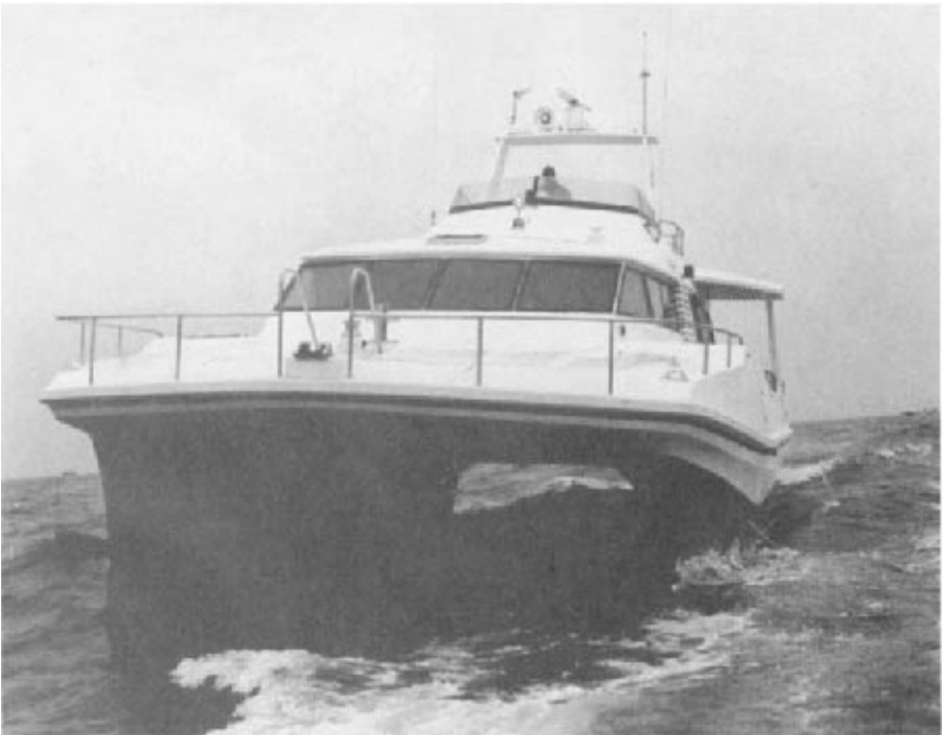
Fig. 9.34 Catamaran with carbon fiber-reinforced hull (courtesy Toray).
