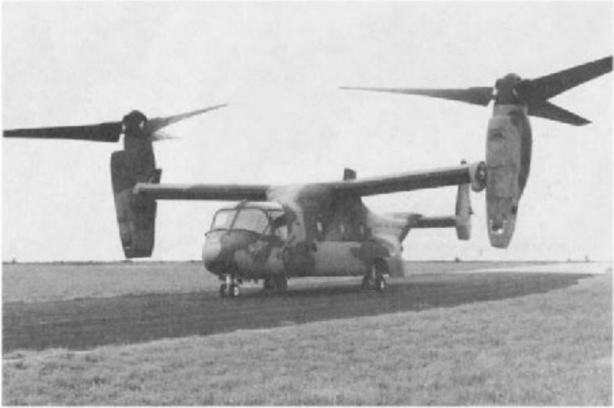
Fig. 9.12 The V-22 Osprey uses polymer matrix composites in the fuselage, wings, empennage, and rotors (courtesy Boeing).
