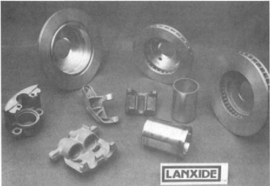
Fig. 9.24 Silicon carbide particle-reinforced aluminum brake rotors, calipers, and other parts provide higher specific stiffness and better wear resistance than monolithic aluminum and are lighter than cast iron (courtesy Lanxide).
