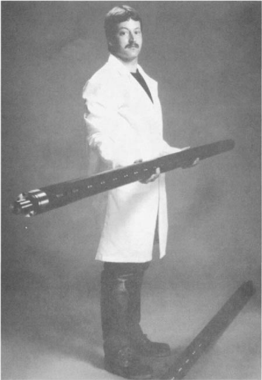
Fig. 9.15 The lower weight of carbon/epoxy rollers used in printing, paper, and conversion equipment facilitates handling. Lower rotary inertia results in reduced tendency to tear paper and plastic film during startup and shutdown (courtesy Du Pont).
