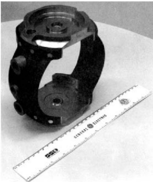
Fig. 9.31 Developmental lightweight, dimensionally stable electro-optical system gimbal composed of parts made from two types of carbon fiber-reinforced epoxy and from silicon carbide particle-reinforced aluminum.
