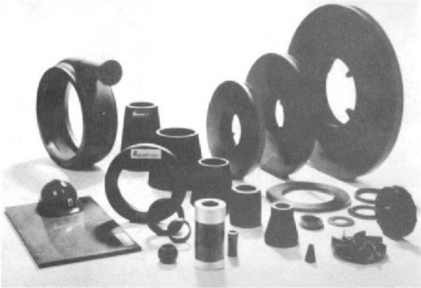
Fig. 9.27 Silicon carbide particle-reinforced alumina ceramic matrix composite parts for wear-resistant applications, including impellers, pipeline chokes and liners for pumps, chutes, valves, and hydrocyclones (courtesy Lanxide).
