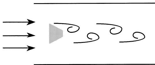
FIGURE 4.23.10 Vortices shedding off a body placed in a moving stream.
