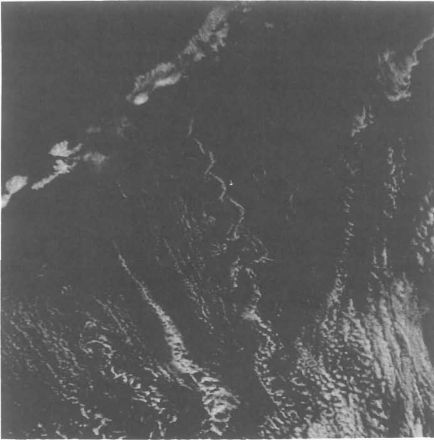
Figure 10.18 A von Karman vortex street downstream of mountain peaks in a strongly stratified atmosphere. There are several mountain peaks along the linear, light-colored feature running diagonally in the upper left-hand corner of the photograph. North is upward, and the wind is blowing toward the southeast. R. E. Thomson and J. F. R. Gower, Monthly Weather Review 105 : 873–884, 1977, and reprinted with the permission of the American Meteorological Society.
