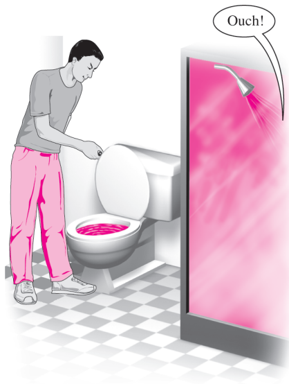
FIGURE 8-50 Flow rate of cold water through a shower may be affected significantly by the flushing of a nearby toilet.
