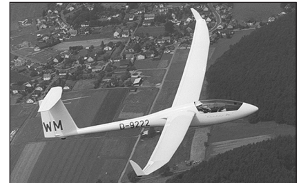
(b) Winglets are used on this sailplane to reduce induced drag.
