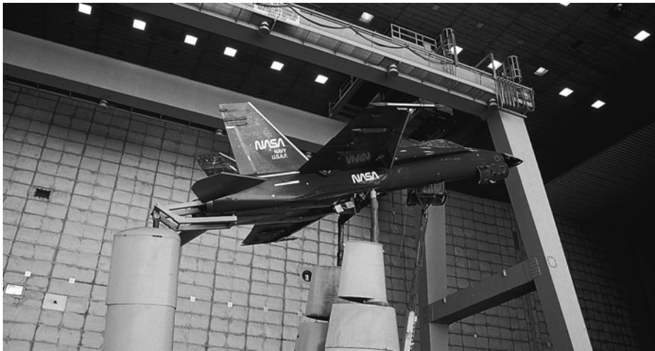
Wind tunnel test of an F-18 fighter plane model. Testing of models is imperative in the design of complex, expensive fluids-engineering devices. Such tests use the principles of dimensional analysis and modeling from this chapter. (Courtesy of Mark E. Gibson/Visuals Unlimited)
