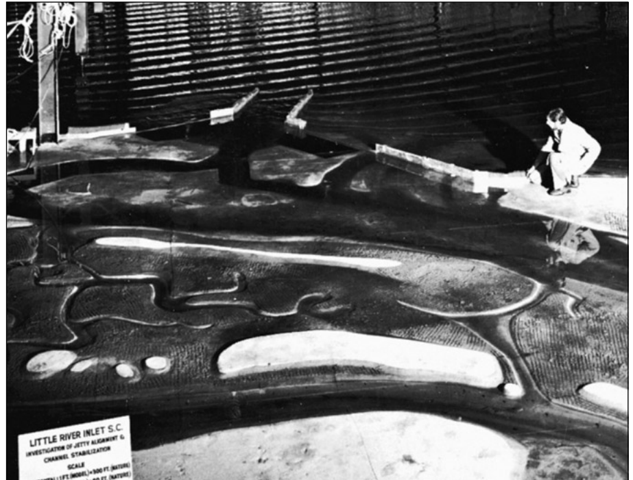
Fig. 5.9 Hydraulic model of a barrier-beach inlet at Little River, South Carolina. Such models of necessity violate geometric similarity and do not model the Reynolds number of the prototype inlet. (Courtesy of U.S. Army Engineer Waterways Experiment Station).
