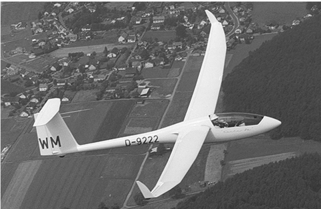
(b) Winglets are used on this sailplane to reduce induced drag. (Courtesy Schempp-Hirth)
