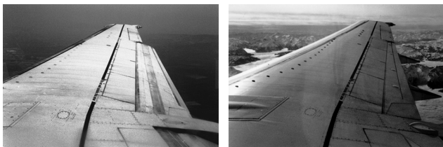
(a) Flaps extended (takeoff) (b) Flaps retracted (cruising)
