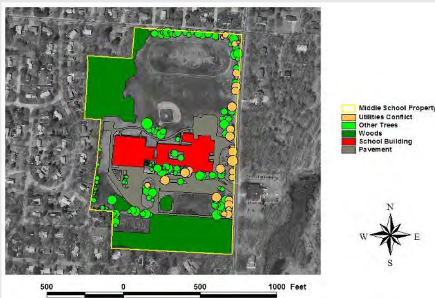
FIGURE 8.5 Trees conflicting with utility lines.
