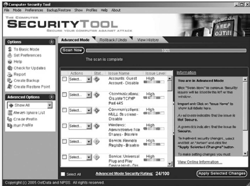
Figure 23-2. A computer security program can identify weaknesses in your operating system's default settings and correct them automatically.
