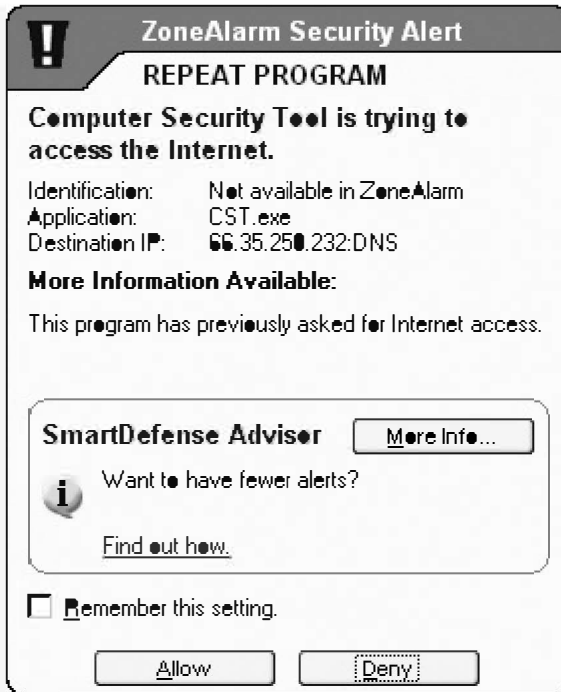
Figure 23-3. Some firewalls ask (annoy) you every time an unfamiliar program tries to access the Internet.
