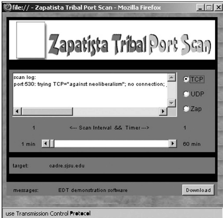
Figure 16-4. The Zapatista Tribal Port Scanner can bombard a target computer's ports with text messages.
