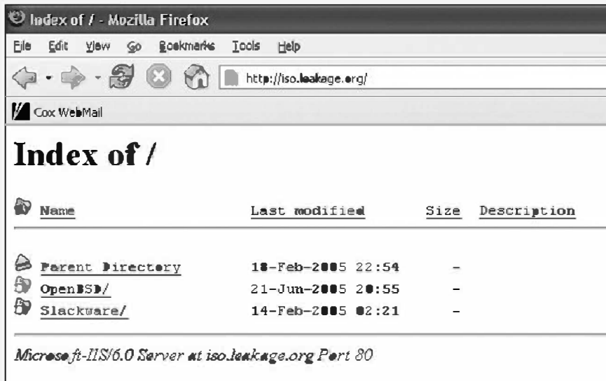
Figure 8-6. A website's directory listing exposes both the directories where crucial files are stored along with the name and version number of the webserver software.
