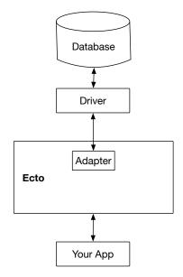
We start at the database, where the raw data is stored. Next, we have the driver, which handles converting values from the database into Elixir. Drivers are database-specific: there's an Elixir driver for Postgres, another for MySQL, and so on.
