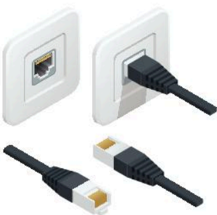
Figure 11.5.1 Ethernet socket and cable
