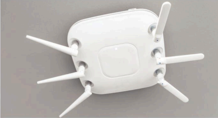
Figure 20.1.1 A WAP is connected to the network by a cable, but computers can connect to the WAP wirelessly, without a cable
