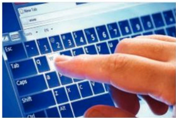
Figure 2.2.2 A touchscreen is an input and an output device combined.
