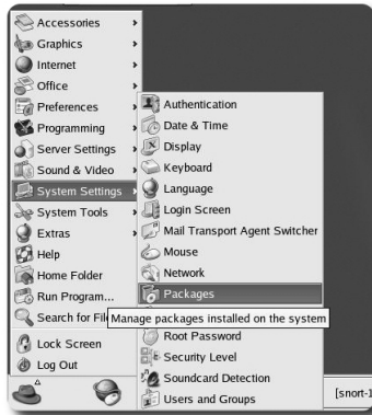
Figure 3.3 Selecting the Packages Utility from the Panel Menu
