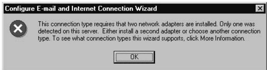
Figure 3.8 Network Interface Card Requirement Warning
