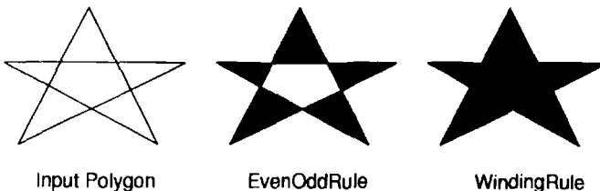
Figure 8.3. Ambiguity in the definition of the interior of a self-intersecting polygon.
