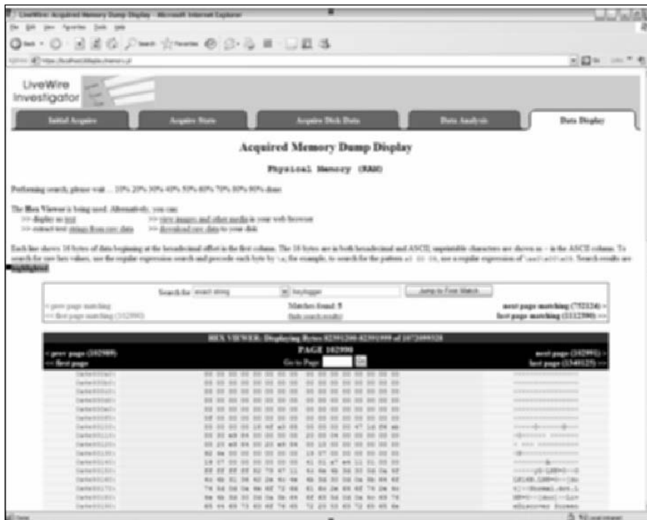
Figure 5.13 A Keyword Search for the Term Keylogger in a Memory Dump Using Wetstone's LiveWire
