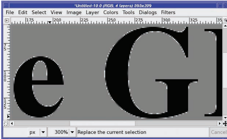
Figure 9-18. Light speckles left behind when you try to use Select by Color on antialiased text
