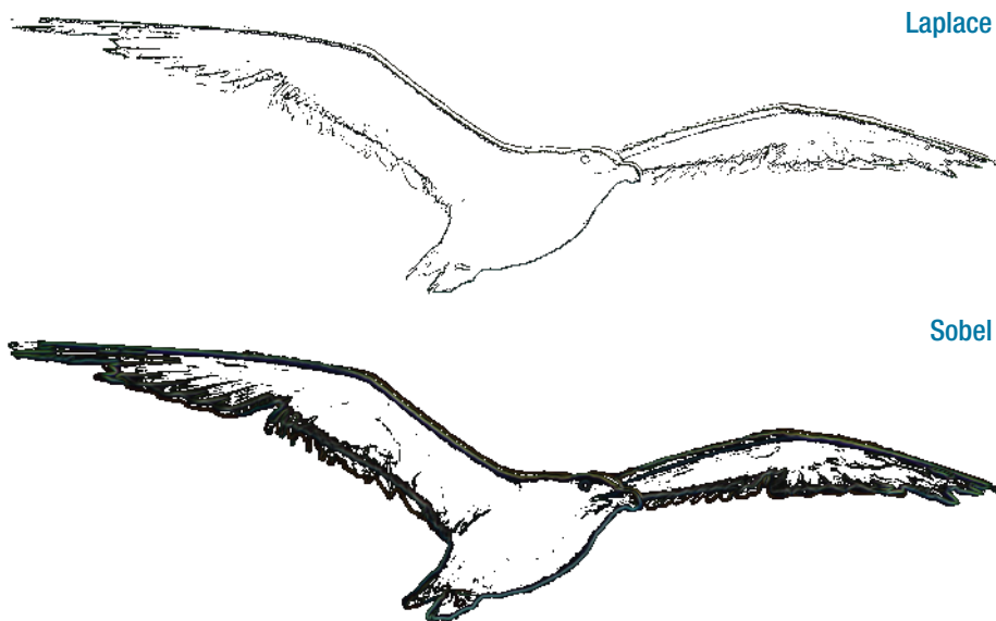
Figure 7-14. Laplace and Sobel are two ways of finding the edges in an image.
