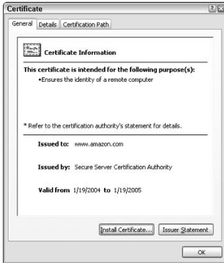
Figure 10-10: Before entering a credit card on a site, make sure the site's certificate contains the site's name and that the date is still valid.
