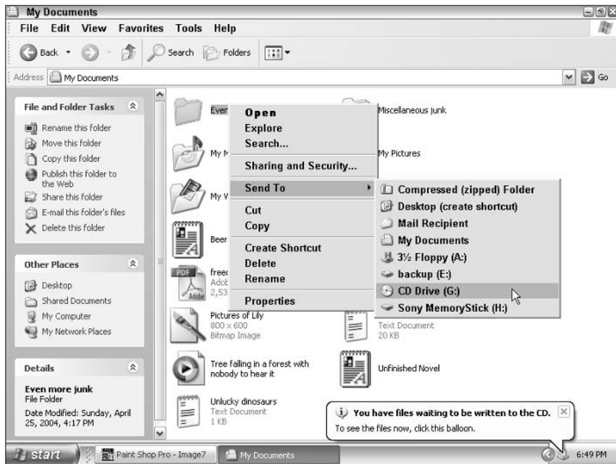
Figure 4-8: Right-click on any files and folders you want to copy to a CD, choose Send To, and select your CD burning drive.
