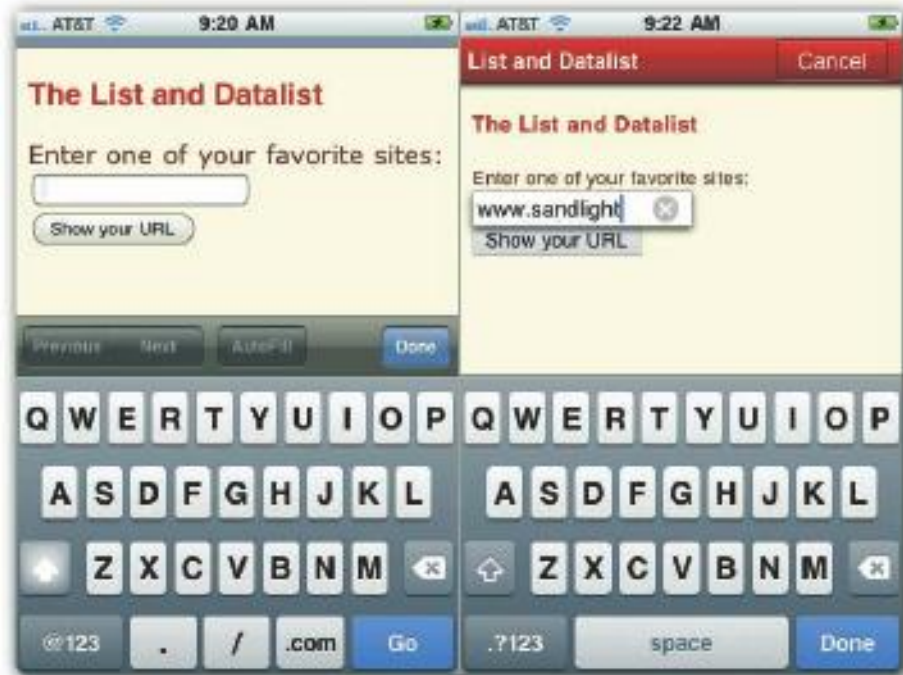
Figure 14-4: Special mobile device keyboard for URL form (left) and standard mobile keyboard (right).
