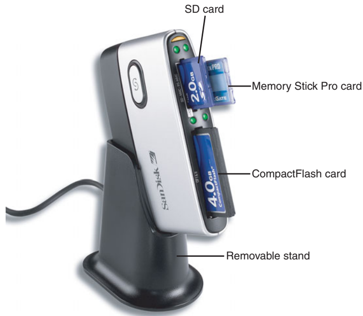
Figure 10.3 The SanDisk 12-in-1 Card Reader/Writer plugs into a Hi-Speed USB (USB 2.0) port and features a removable stand. (Photo courtesy of SanDisk.)
