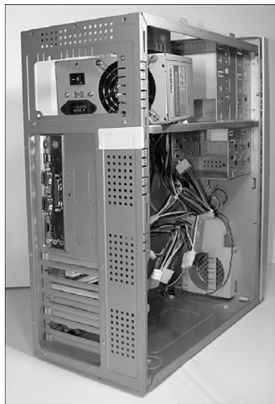
Figure 19.16 Installing the power supply into the chassis.
