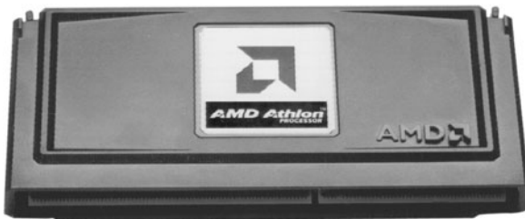
Figure 3.42 AMD Athlon processor for Slot A (cartridge form factor).
