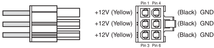
Figure 18.35 PCI Express x16 Graphics 6-pin power connector.
