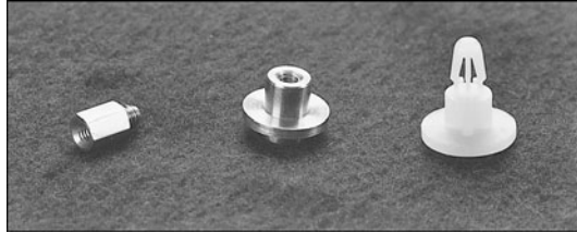
Figure 19.10 Various types of motherboard standoffs, used to support the board when installed in the chassis or motherboard tray.
