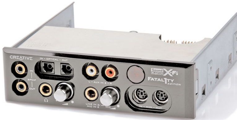
Figure 13.2 An internal breakout box providing support for MIDI in/out, coaxial and digital SPDIF in/out, convenient volume control knobs, stereo out, headphone out and line in jacks, and support for an IR remote control.
