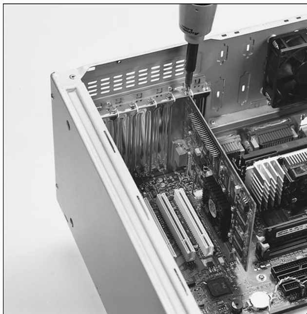
Figure 19.25 Installing the screw to retain the card.
