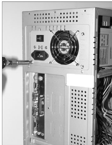
Figure 19.17 Installing the screws to retain the power supply.
