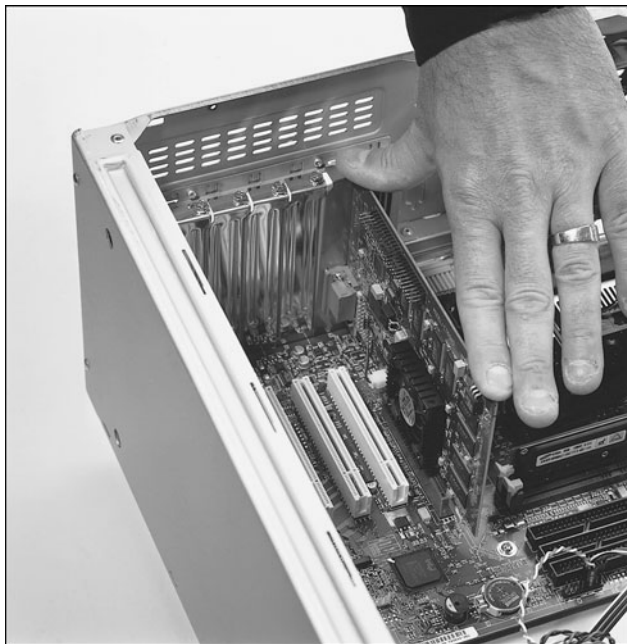
Figure 19.24 This photo shows a video adapter being inserted into the slot.
