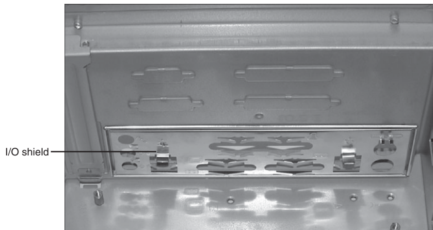
Figure 19.13 The I/O shield after being snapped into place in the chassis.
