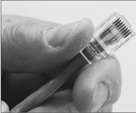
Figure 17.14 Push the RJ-45 connector into place, ensuring the cable pairs are ordered properly.
