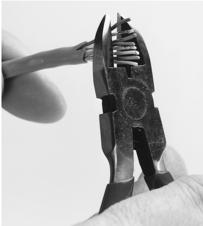
Figure 19.20 An even trim and proper stripping of the UTP cable is essential to a good RJ-45 cable.
