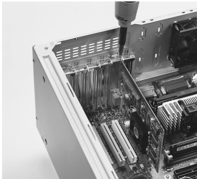
Figure 24.26 Installing the screw to retain the card. Video card courtesy of Creative Labs, Inc. Motherboard courtesy of Intel Corporation.
