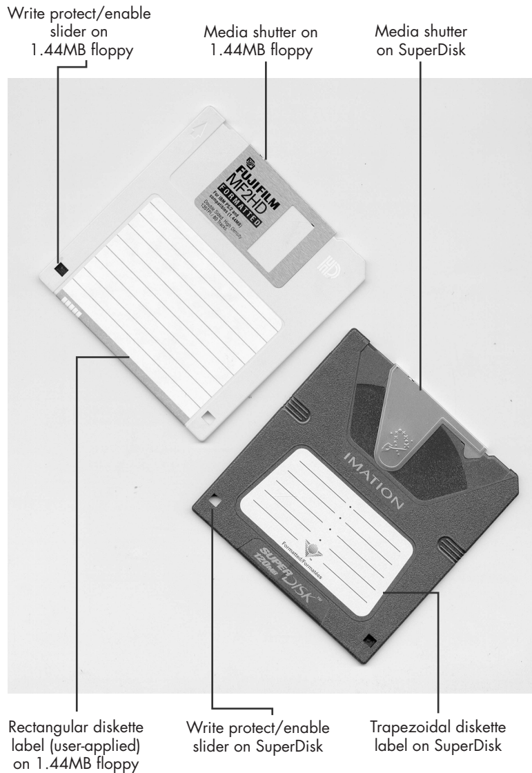
Figure 12.1 A standard 1.44MB 3.5-inch floppy diskette (top) compared to LS-120 SuperDisk media (bottom).
