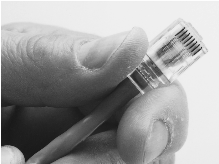
Figure 19.21 Push the RJ-45 connector into place, ensuring the cable pairs are ordered properly.
