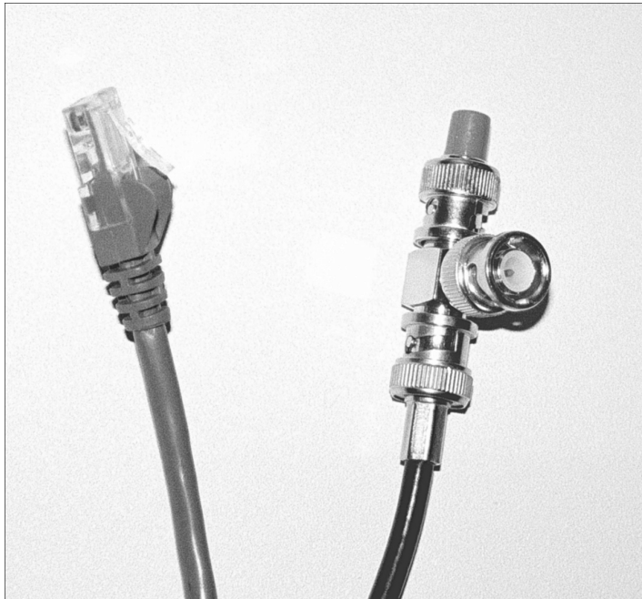
Figure 19.6 An RJ-45 UTP cable (left) and a Thin Ethernet cable with BNC T-adaptor and terminator (right).
