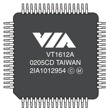
Figure 16.8 The VIA VT1612A is a typical AC'97 2.2-compliant codec chip. Photo courtesy of VIA Technologies, Inc.
