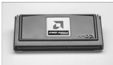
Figure 3.54 AMD Athlon processor for Slot A (cartridge form factor).
