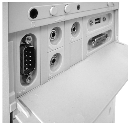
Figure 23.29 FrontX 5.25" bay casing with several ports installed. Photo courtesy FrontX.com.
