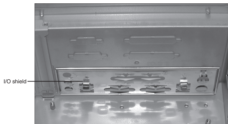
Figure 22.16 The I/O shield after being snapped into place in the chassis.
