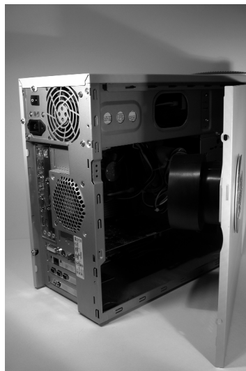
Figure 23.27 Side cover with the duct being reinstalled on the chassis.
