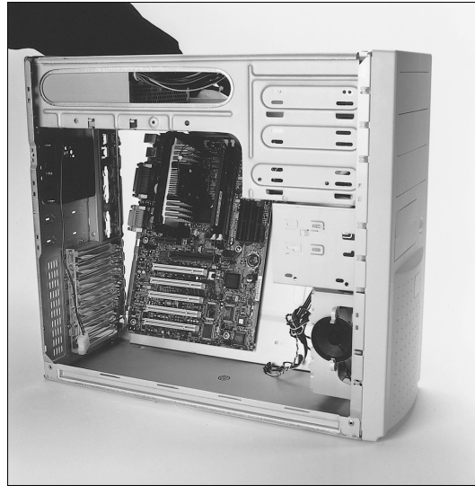
Figure 22.17 Installing a motherboard and tray into the chassis. Case courtesy of PC Power & Cooling, Inc. Motherboard courtesy of Intel Corporation.
