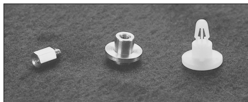
Figure 22.12 Various types of motherboard standoffs, used to support the board when installed in the chassis or motherboard tray.
