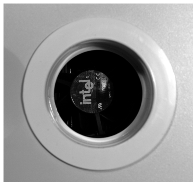
Figure 23.26 Peering through the duct to measure the clearance between the duct and processor heatsink.
