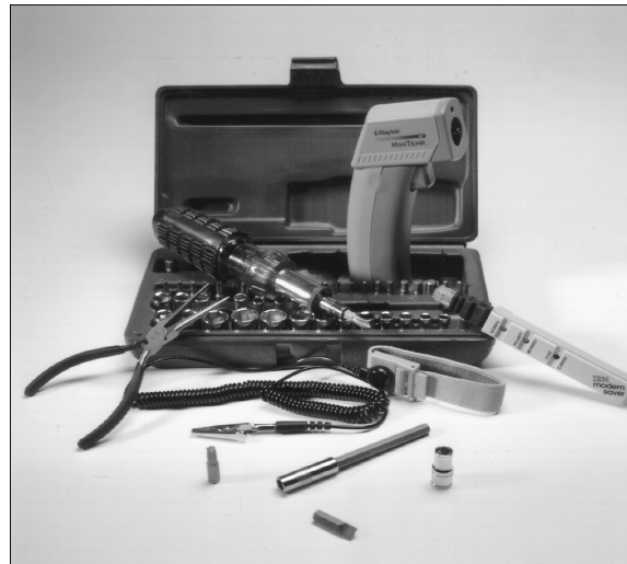
Figure 24.2 The basic tools you need to work on your PC are shown here.
