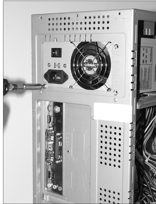
Figure 22.20 Installing the screws to retain the power supply.
