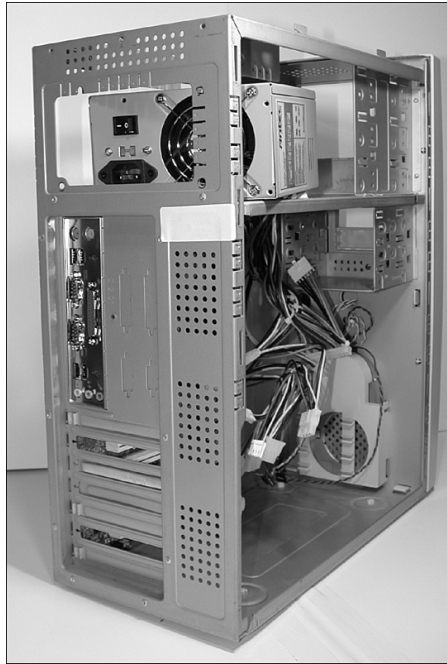
Figure 22.19 Installing the power supply into the chassis.
