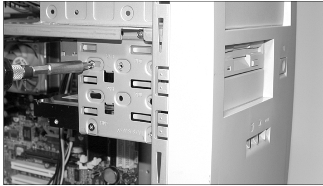
Figure 22.25 Use four screws to secure each drive to the drive bay. If your computer uses a removable drive cage, mount the drives to the drive cage in the same way.
