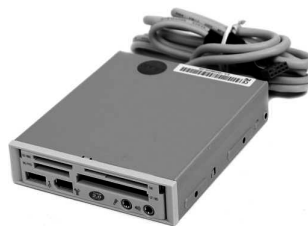
Figure 23.30 In-Win CR-I530 3.5" bay USB/FireWire/audio plus digital card reader. Photo courtesy NewEgg.com.
