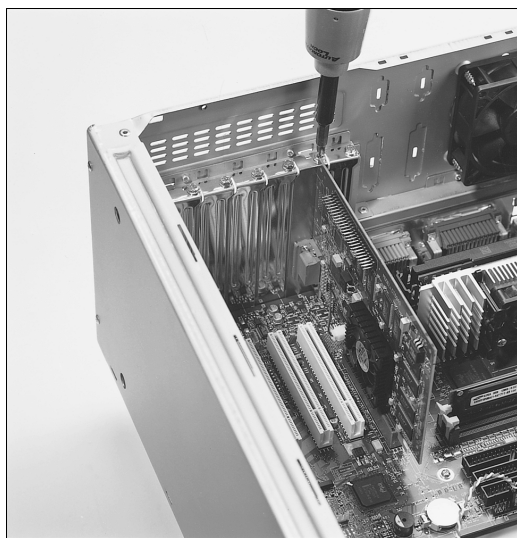
Figure 22.28 Installing the screw to retain the card. Motherboard courtesy of Intel Corporation.
