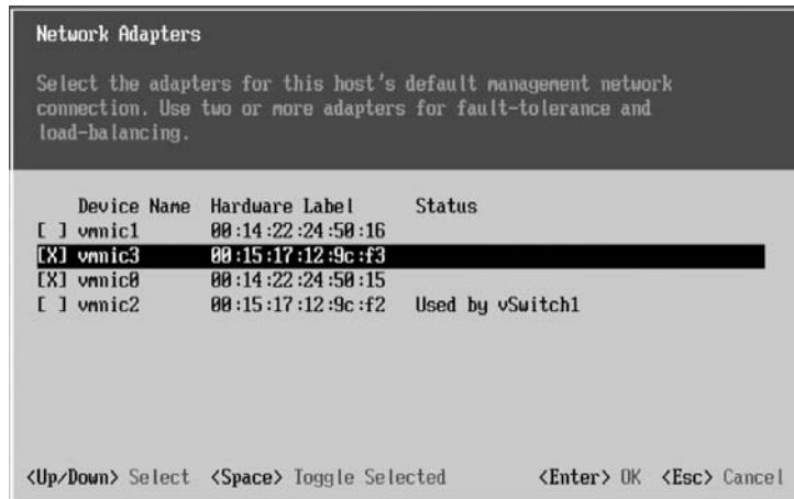
FIGURE 13.13 One or more network adapters can be selected for the host's default management network.
