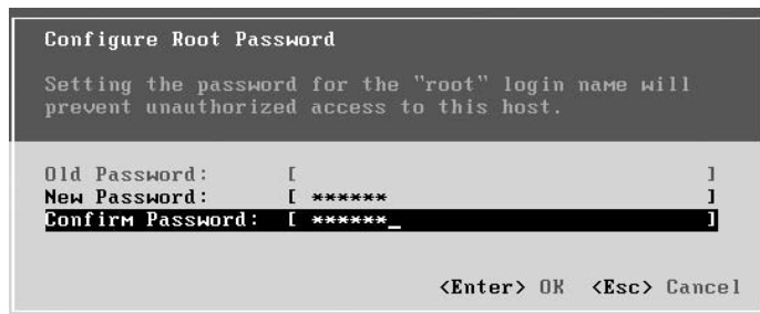
FIGURE 13.9 Change the root password upon first boot of the ESXi thin hypervisor.
