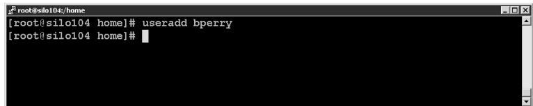
FIGURE 12.31 Create the local Ser- vice Console account that matches the name in AD.
