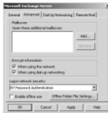
Figure 7.19 Enabling Encryption for Outlook MAPI over RPC Clients
