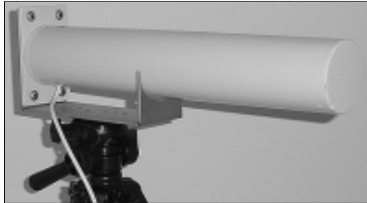
Figure 15.3 Yagi Antenna on a Tripod Mount
