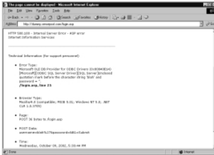
Figure 11.10 Error Returned to the Browser After Injecting blah and a Single Quote
