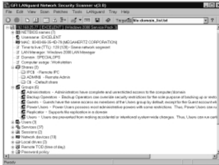
Figure 5.25 Viewing a Scan Output with GFI LANguard Network Security Scanner
