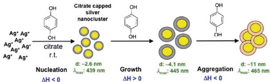
Fig. 6 Illustration of the growth mechanism for AgNP synthesized using HQ at room temperature as proposed in Ref. [32]. Change color in NP shell indicates HQ replaced citrate as capping agent
