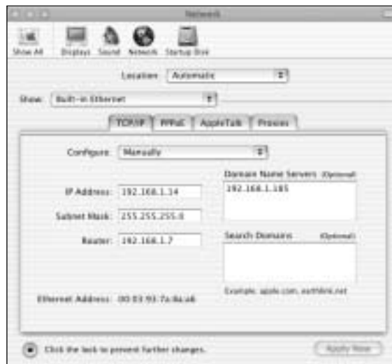
Figure 5.10 You can use the GUI to find out your Ethernet address with an OS X system.
