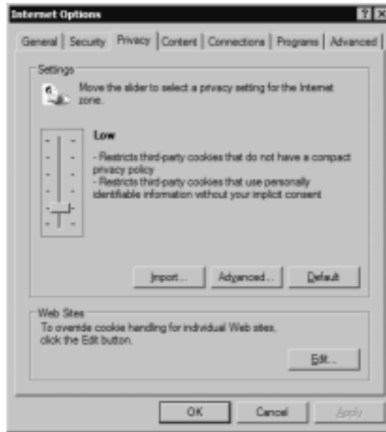
Figure 8.2 Cookie options can be set in IE via the Privacy tab in Internet Options.
