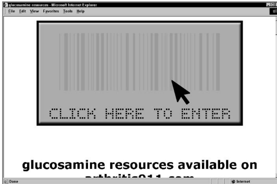
Figure 7-3: The mouse pointer triggers a JavaScript mouseover event on the image, loading another page.
