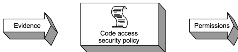
Figure B.1 The CLR code access security policy takes the assembly evidence as input and produces a permission set as output.
