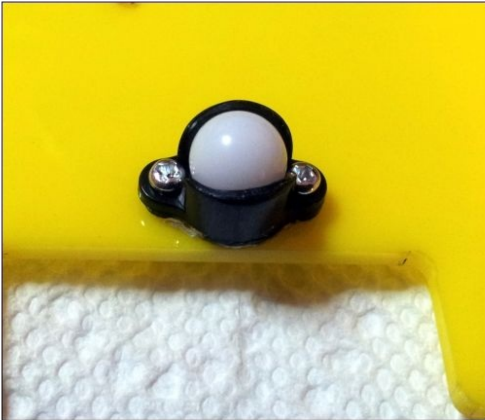
Mounting the castor wheel
