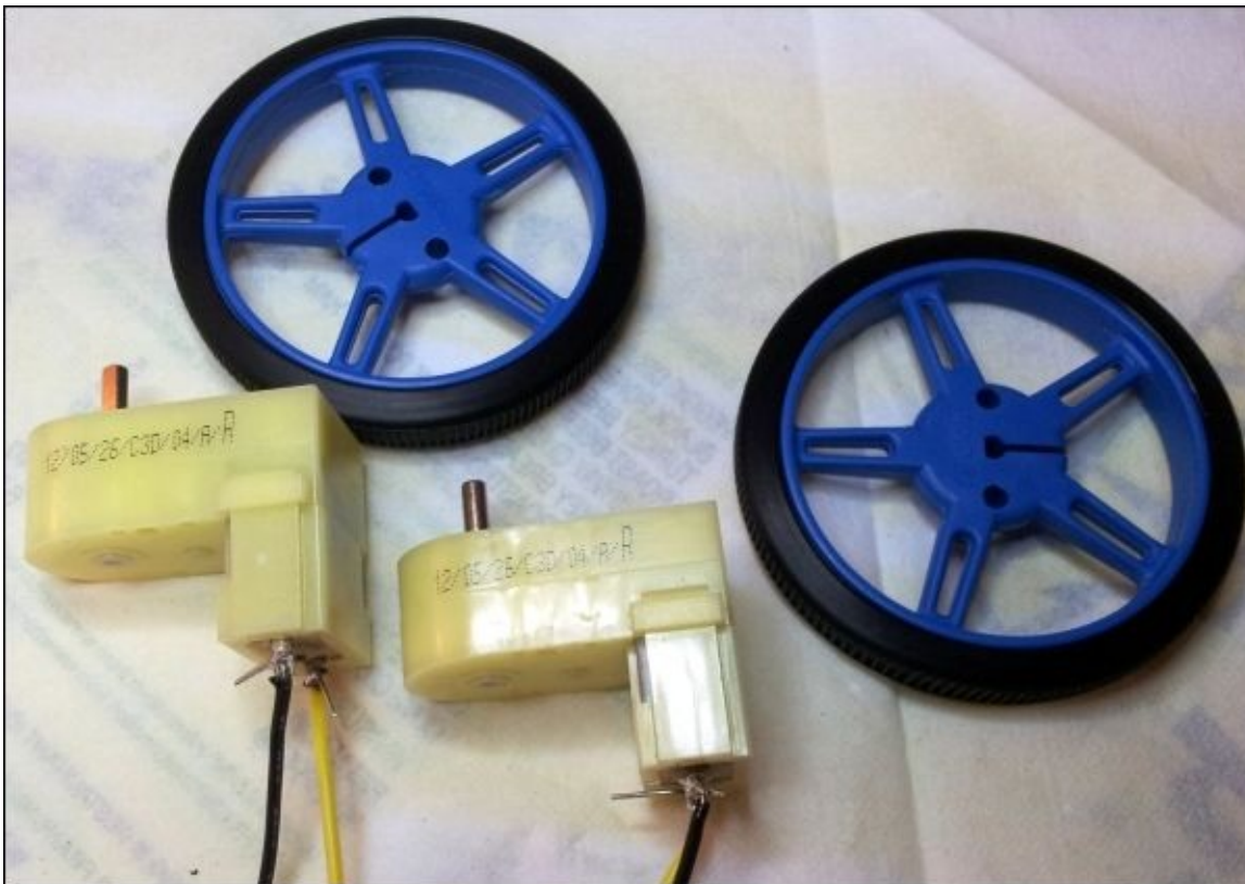
DC motors with soldered wires and wheels with strapped silicone tires
