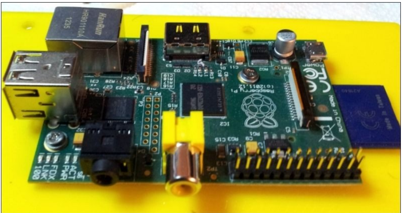
Raspberry Pi mounted using M2.5 screws
