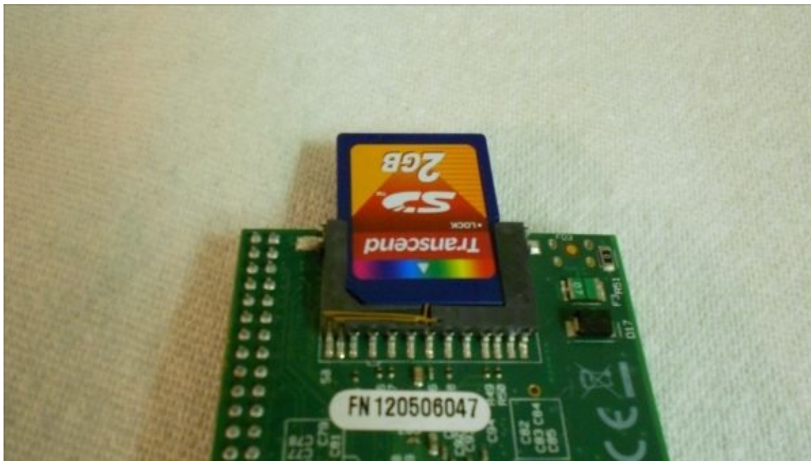
A flashed SD card in the slot
