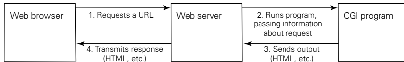
Figure 1.3 To respond dynamically, a web server can spawn a CGI program to handle a web request.
