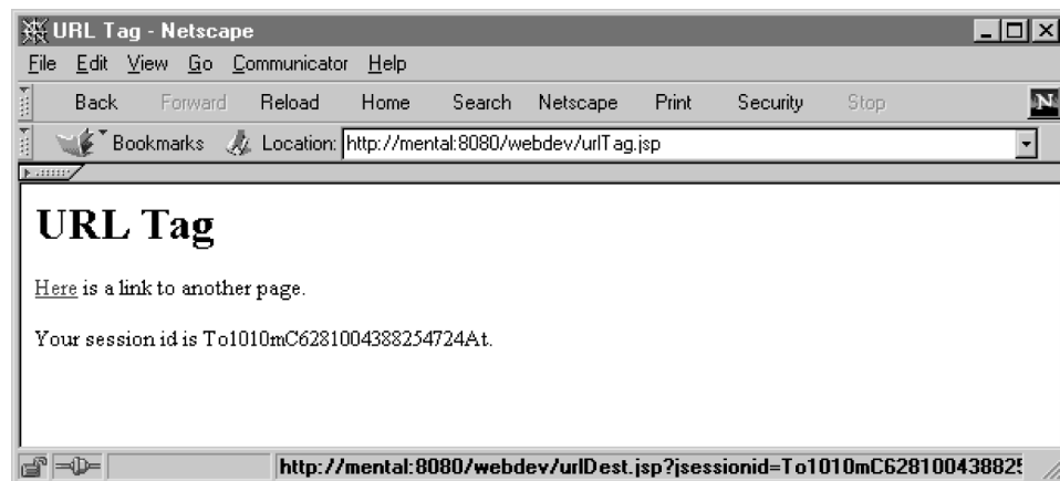
Figure 18.10 Output of URL rewriting tag for the first request, and all requests when cookie support is disabled
