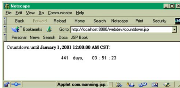
Figure C.2 Countdown applet running via <jsp:plugin> tag
