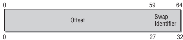
Figure 18-6: Components of an architecture-independent swap identifier.
