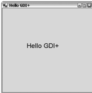
Figure 11-2. The rendering results if the base OnPaint is placed last in the method
