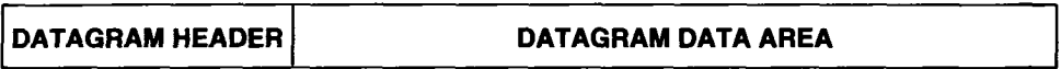
Figure 7.2 General form of an IP datagram, the TCP/IP analogy to a network frame. IP specifies the header format including the source and destination IP addresses. IP does not specify the format of the data area; it can be used to transport arbitrary data.
