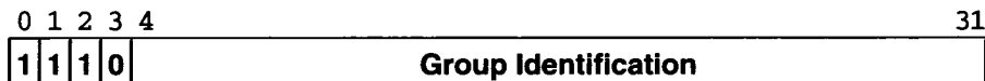
Figure 17.1 The format of class D IP addresses used for multicasting. Bits 4 through 31 identify a particular multicast group.
