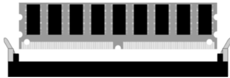
Figure 2-2: Align a DDR module with its socket.
