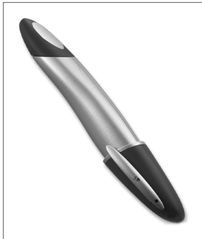
Figure 2-5: A digital pen is a specialized scanner.
