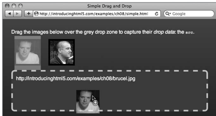
FIGURE 8.1 All images and links are draggable by default. With a little more code, you can make them droppable too.
