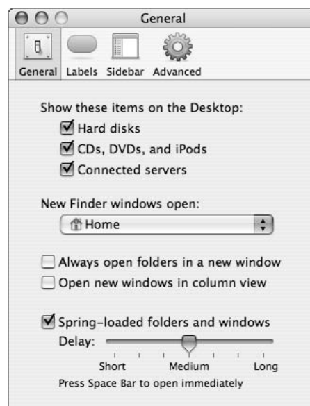
• Figure 16-9: Use the Finder's preferences to dictate what volumes are mounted on the Desktop.
