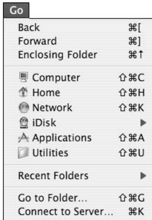
• Figure 9-1: The Go menu can help you navigate with the mouse, and it lists the keyboard equivalents.
