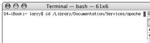
• Figure 56-16: Dragging a folder into the Terminal copies that folder's path there.
