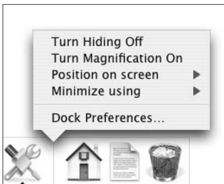
• Figure 13-8: You can adjust the Dock's preferences from the Dock's contextual menu.
