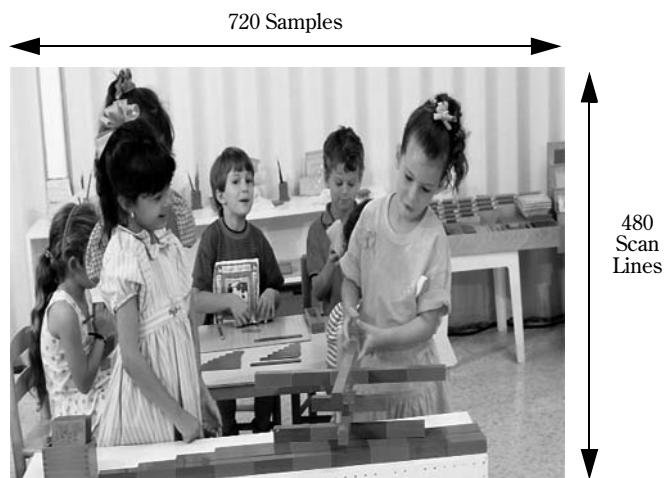
Figure 7.33. Scaling 16:9 Content for a 4:3 Display: "Squeezed" mode. Entire 16:9 program horizontally squeezed to fit 4:3 display, resulting in a distorted picture.
