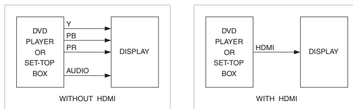
Figure 6.48. Using HDMI Eliminates Confusing Cable Connections For Consumers.
