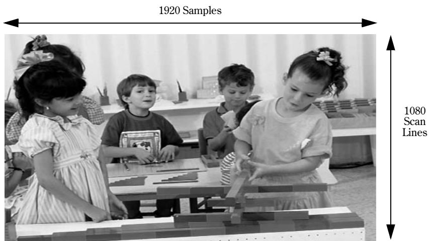
Figure 7.36. Scaling 4:3 Content for a 16:9 Display: “Wide” mode. Entire picture linearly scaled horizontally to fill 16:9 display, resulting in distorted picture unless used with anamorphic content.
