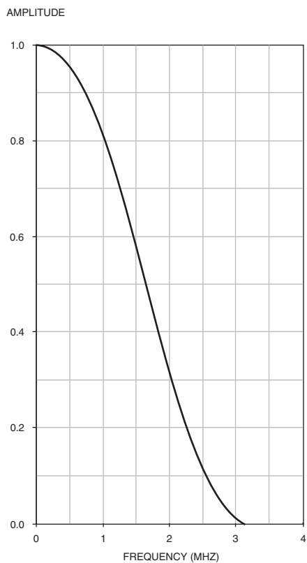
Figure 9.26. Typical 1.3-MHz Lowpass Digital Filter Characteristics.
