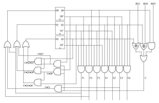
We need to back check the don't care states to see that the machine will not get trapped. It turns out that for C=0, the unused state will jump to F0 (000), and if C=1 it will jump to E2 (110). This is probably acceptable. In any case it should not be a problem as we will definitely need to add some extra hardware to force the processor to do a particular operation at start up. In practice this will be a jump to the start of a stored program in ROM, which will load a minimal operating system.
