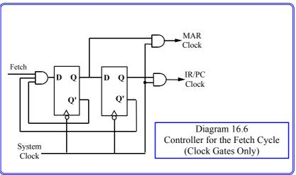
state we can implement the output logic trivially as shown in Diagram 16.6. The clocks to the MDR and RAM chips are blocked during the fetch cycle, and the multiplexers are both given a zero control input.
