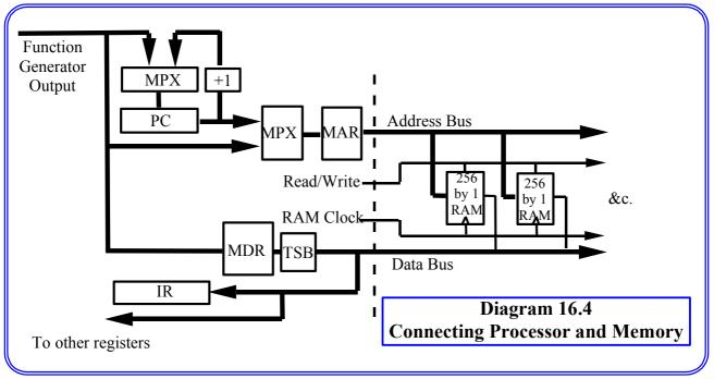
instructions (as opposed to data) from the memory. These are called the Program Counter (PC) which stores the address of the next program instruction to be executed, and the Instruction Register, which will act as a store for the program instructions. The IR will be decoded to determine the function of the central processor. The arrangement is shown in Diagram 16.4. Since we have opted to use 256×1
