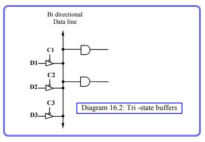
but is effectively disconnected from the data line. It is the logic designers problem to ensure that no two circuits feed the data line at the same time.
