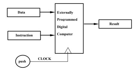
Before we can design the workings of the externally programmed digital computer, we need to define the **external interface** : **Data** is 8 bits wide
