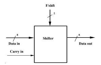
The two function selection bits can specify four different functions; there are three obvious ones: **unchanged**, **shift right**, and **shift left**. However, there are two different types of shift right functions. The **logical right shift** function shifts in a logic **0**
