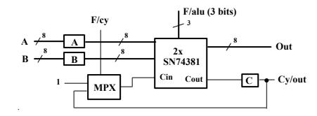
The carry bit applied to the arithmetic unit can now come for two sources. It may be a logic 1, or the carry bit stored in the C register which was left there during the last operation. This arrangement looks rather arbitrary, the idea behind it is that it is not difficult to produce a zero bit in the C register by the selection of the appropriate ALU function. Thus, the bit can be selected either a 0 or a 1 through the multiplexer.
