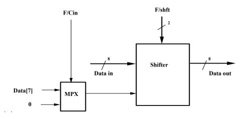
For left shift we may want  $\mathbf{0}$  (for both arithmetic and logical left shift functions) or possibly an independent carry input bit. We would need a second multiplexer for this or a four-input one output multiplexer. We select the latter one and arrive at our final shifter circuit:
