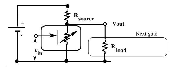
In this model the output does not change instantaneously like a switch; however,  $V_{out}$  vs  $V_{in}$  (as shown in the next diagram) is not a linear function. The output vs. input voltage of a given configuration (with a given  $R_{load}$ ) will have the form:
