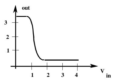
We can see that the output remains relatively high (around 3.5 volts) as long as the input voltage is below 1 V. When the input voltage is above 1.5 V then the output is already very low, near to zero, in practice it is near to 0.3V. In fact, this model is closer to the actual physical truth because physical voltage signals cannot change instantaneously.
