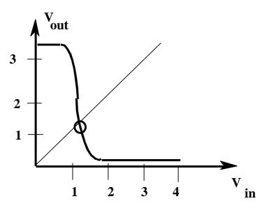
The fascinating thing is that in the laboratory either output behaviour of an inconsistent circuit can occur. It may oscillate or settle at an **Indeterminate** value.
