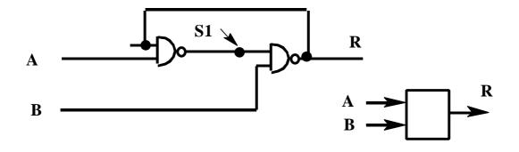
For this method we use the **Delay Model**. The first step is to give a signal name to all inputs and outputs. The signals **A**, **B**, and **R** have been specified with the circuit, we use the symbol **S1** for the output of the first **NAND** gate.
