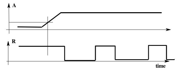
We have not finished yet. What kind of behaviour will our second model give us? When the **A** input of the **NAND** gate is set to **Logic-1** the device becomes a one-input, one-output inverter. We can use feedback to connect this output to the input and in fact we have the simple equation for the inverter:
