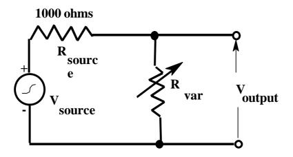
Electrical engineers learn **Ohm's law** early in their student carrier and can tell you that the output  $V_{output}$  can be calculated by:
