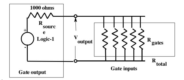
Our electrical engineering friend tells us that the combined resistor value of "N" resistors connected in parallel is:
