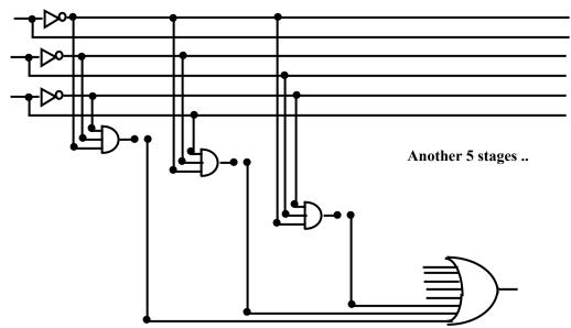
This is called a **Programmable Array Logic (PAL)** device and for the three-input circuit has eight three-input **AND** gates (the number of possible functions) and one eight-input **OR** gate.
