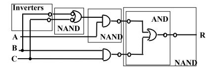
We can do this by applying DeMorgan's formula; i.e. (A'+B')' = AB. However, we do not have to go back to the Boolean equation, we can do this gate transformation operation on the circuit diagram, as shown above. We introduce two inverters (which cancel each other) at the appropriate places in the circuit and transform the gates accordingly.
