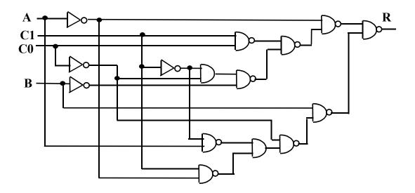
Counting gates, we have to use nine NAND, two AND and four Inverter gates and, accordingly, three type SN7400, one type SN7406 and one type SN7408 ICs. The cost would be:
