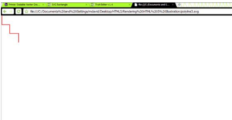
Figure 3.10 A drawing created of straight lines can be created using the POLYLINE element.
