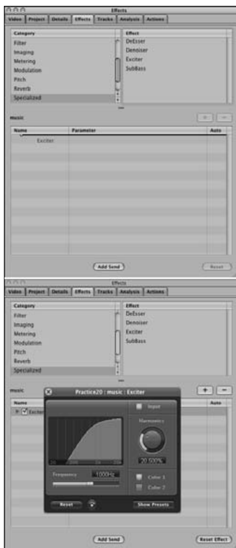
• Figure 19-5: In Soundtrack Pro (or a similar DAW), find an effect and then click and drag it into the window associated with the selected track (top). A control panel for that effect appears (bottom), allowing you to make adjustments to the effect's parameters.
