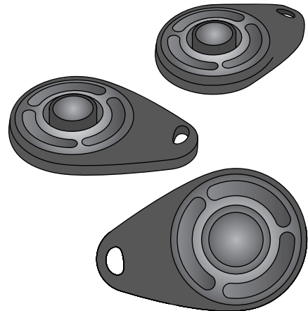
• Figure 15-1: Dog clickers like these create spikes in audio, making edit points (and mistakes) easy to find.
